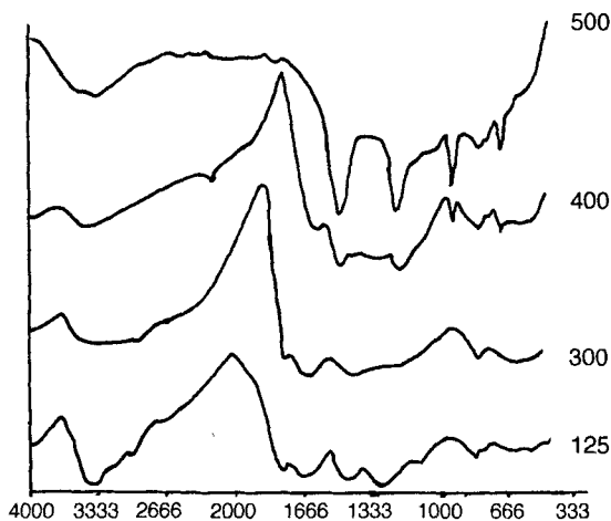
FIGURE 4 The IR spectra of sample D and of residues heated to different temperatures.
